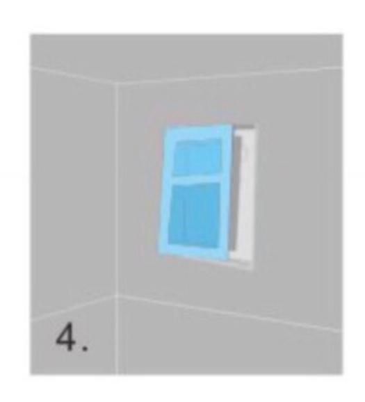
Seal joints between BTS niche and backer board with waterproof sealant.
