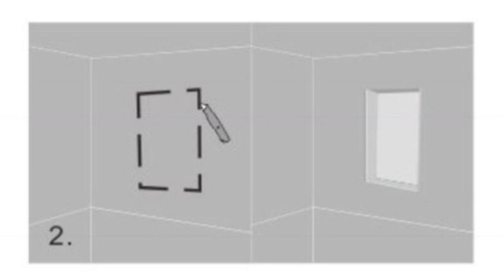
Cut along line and remove top substrate layer if necessary. Install horizontal cross bracing to support BTS niche.
