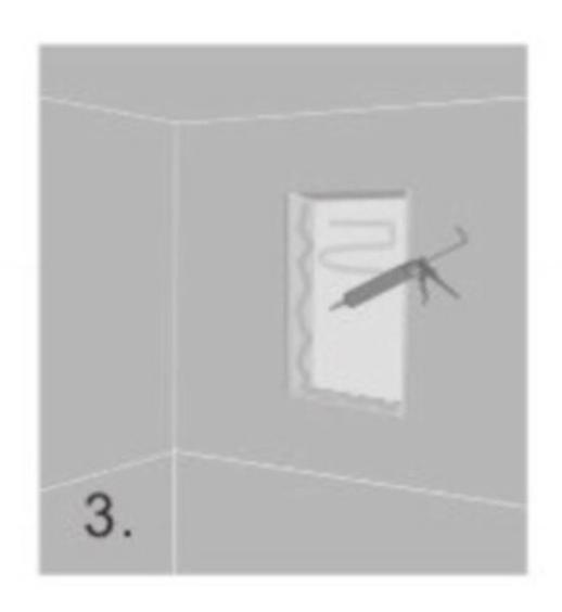
3. Use waterproof sealant to adhere BTS niche to studs.
