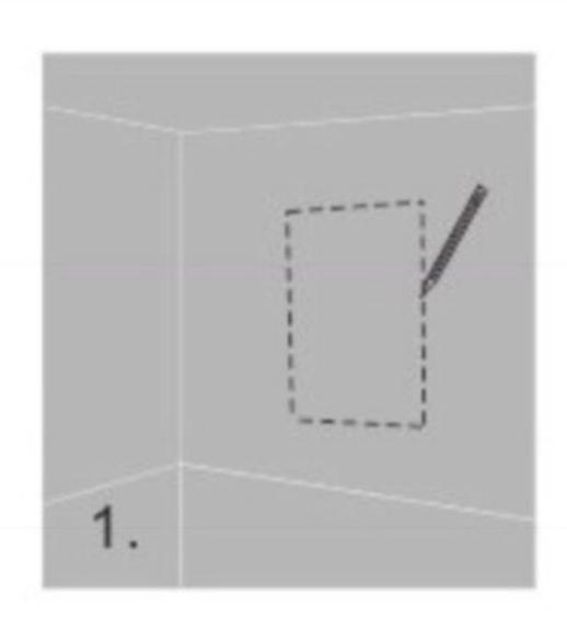
Determine desired height of niche and draw level line on substrate layer. Place BTS niche centered on level line
